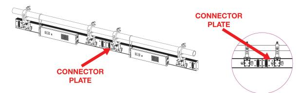
2. Remove the two (2) screws holding the connector plate in place, as well as two (2) screws on the end of each adjacent unit, for a total of six (6) screws. Remove the connector plate.
