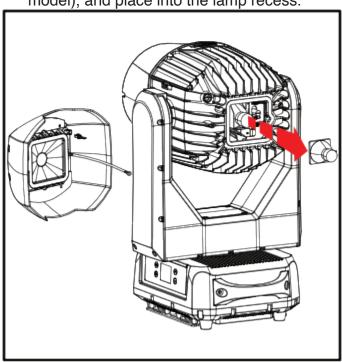
4. Reinstall the head panel, fastening it securely before reapplying power.
