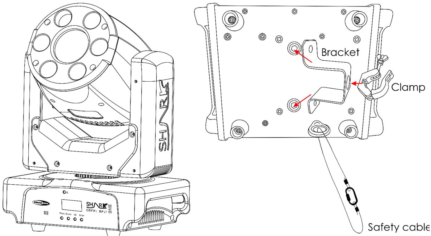
The Shark can be placed on a flat stage floor or mounted to any kind of truss with a clamp.
